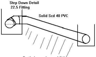
Earth dam - pipe and fitting must be installed so that 4" lateral pipe is 1/2 full before overflow in stepdown occurs.
